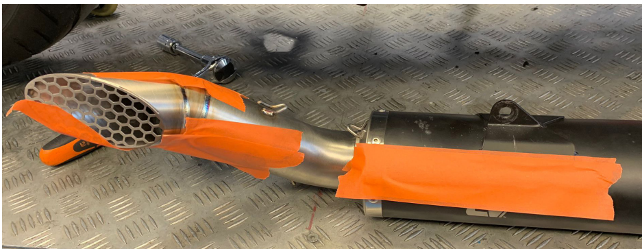
PHOTO 11b - Protect the frame with tape
