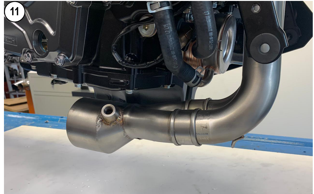
11 SLIDE IN THE SECONDARY PIPE
