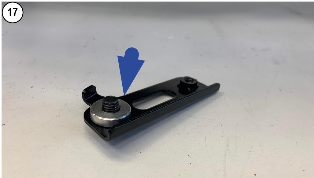
17 PUT THE SPACER ON THE BRACKET IF YOU DON'T HAVE THE UNDER COWL YOU HAVE ALREADY DONE
