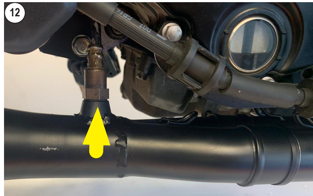
SCREW THE LAMBDA SENSOR
