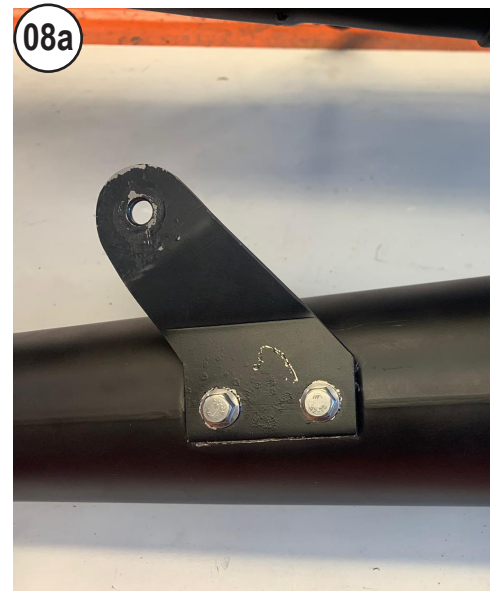
FIT THE LeoVince's BRACKET AT THE MUFFLER
