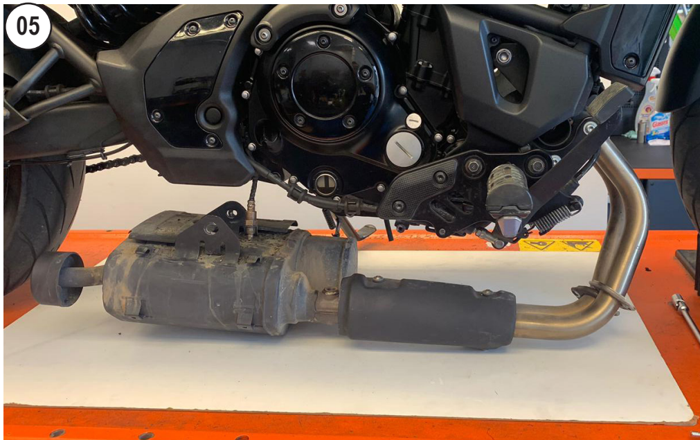
REMOVE THE STOCK EXHAUST
