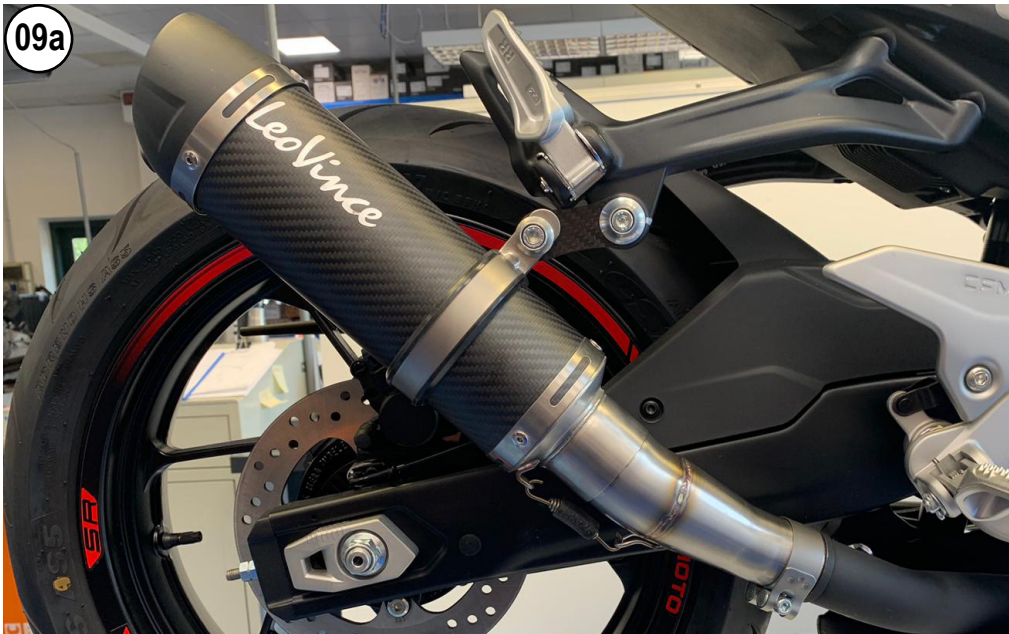
CHECK ALL THE TIGHTENINGS
