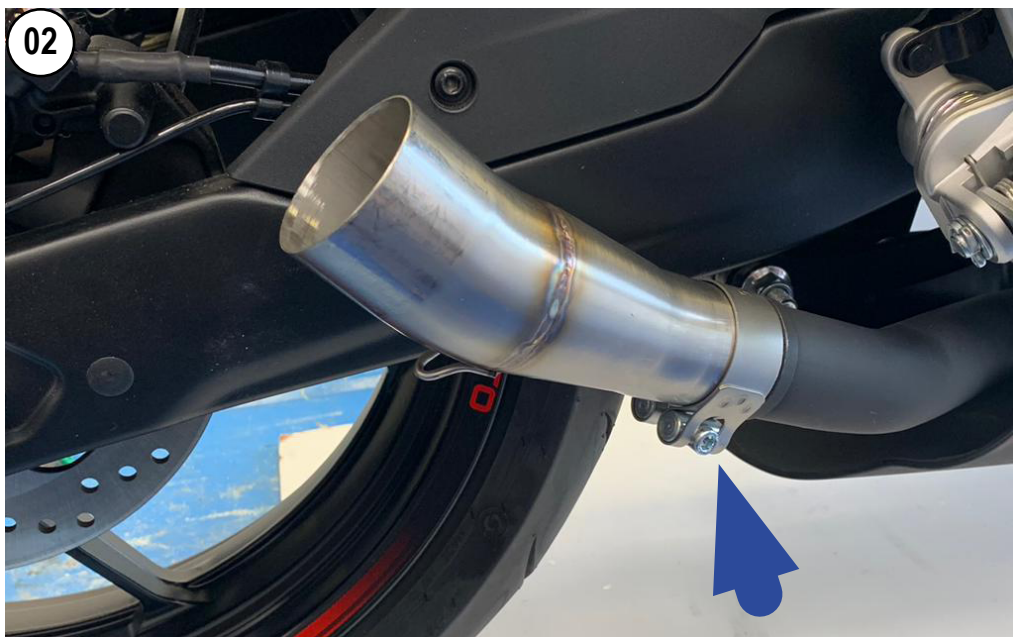
FIT THE CLAMP ON THE PIPE AND INSTALL THE PIPE
